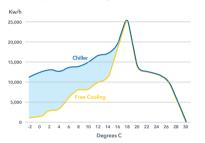
This graph shows the difference between the energy consumption of a free-cooling chiller versus a non-free-cooling variant. When the chiller is operating in free-cooling mode, only the speedregulated fans are consuming energy.
